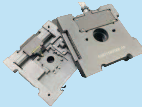
Socket for checking short circuit operation
